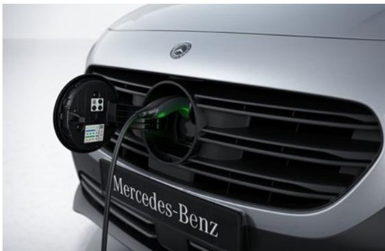
CCS rapid charging port, 75kW max. capacity.
