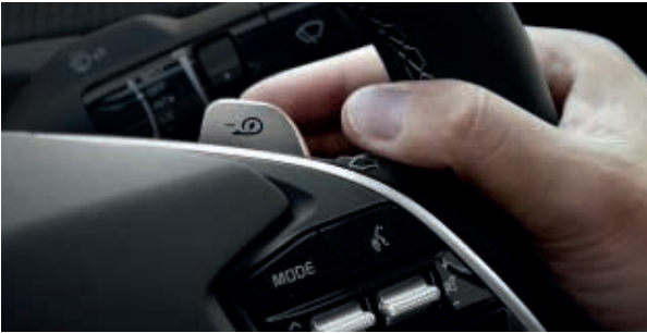
Smart regenerative braking system. This improves the vehicle's range and stability by optimising front and rear-wheel regenerative braking. It can be operated with the steering wheel paddle switches and adjusts the level of regenerative coasting based not only on navigation data, but on radar data as well.
