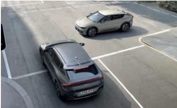
Forward Collision-Avoidance Assist with junction turning and crossing. It uses a front-view camera and radar to detect any vehicles, pedestrians or cyclists ahead. By warning and braking automatically, it can help you avoid, or reduce the severity of an accident. The system also engages when you are crossing or turning at an intersection (grade dependent).
