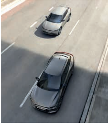
Blind-Spot Collision-Avoidance Assist. When you signal a lane change, you are warned if a risk of collision is detected with a vehicle beside you or approaching from the rear. The system even interacts with your steering if the risk increases. Blind-Spot Collision-Avoidance Assist also watches out for you when pulling out of parallel parking spaces, warning you about oncoming traffic behind you (grade dependent).
