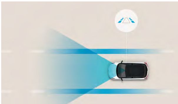
Lane Follow Assist (LFA): Smart sensors and the forward-facing camera detect when the car drifts from the centre of the lane, applying steering torque to maintain road positioning for safety. The car also estimates the trajectory of the vehicle ahead and adjusts its position accordingly.
