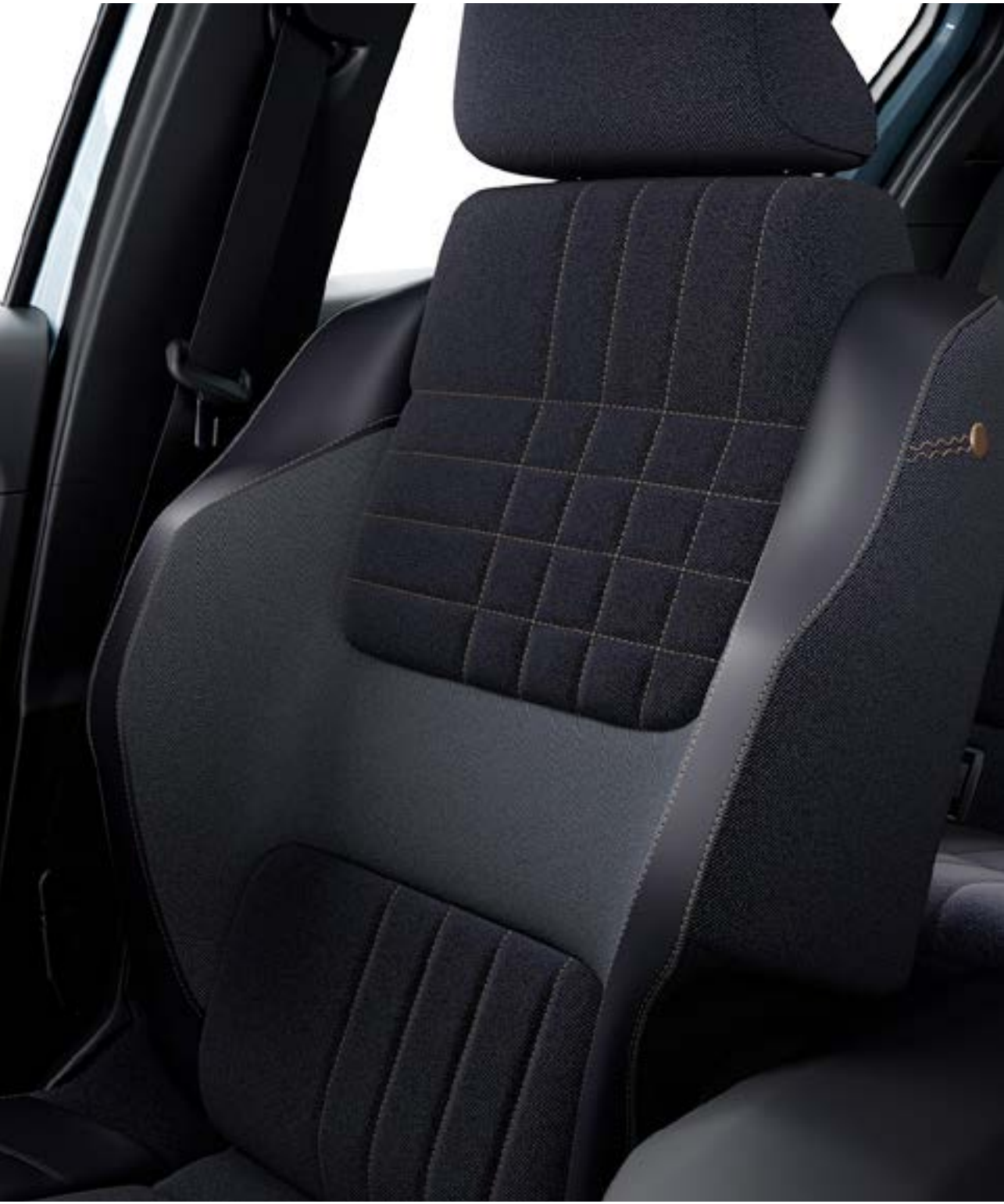
mixed recycled upholstery, quilted "jeans" textile with copper stitching and rivet/ dark blue refined textile
