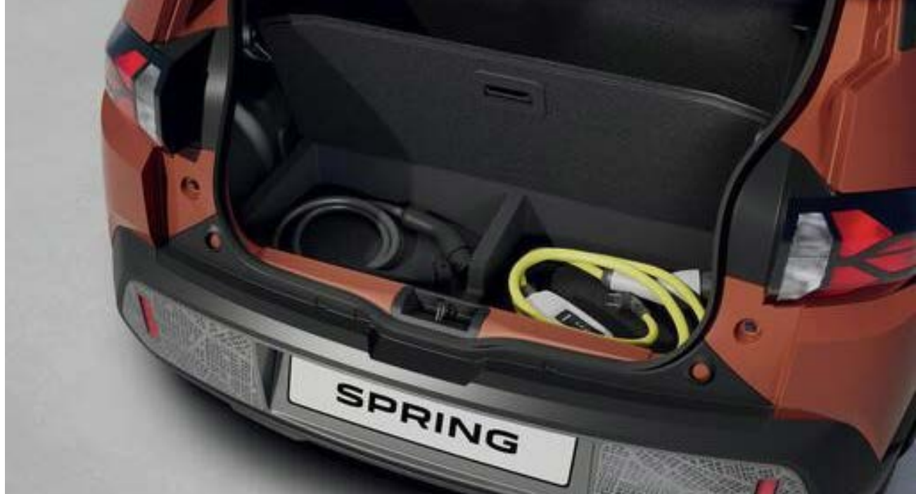
Double floor for cable storage
