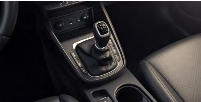
Six speed Intelligent Manual Transmission (iMT) standard on all 48V Mild Hybrid trims. Car shown is not to UK Specification.
