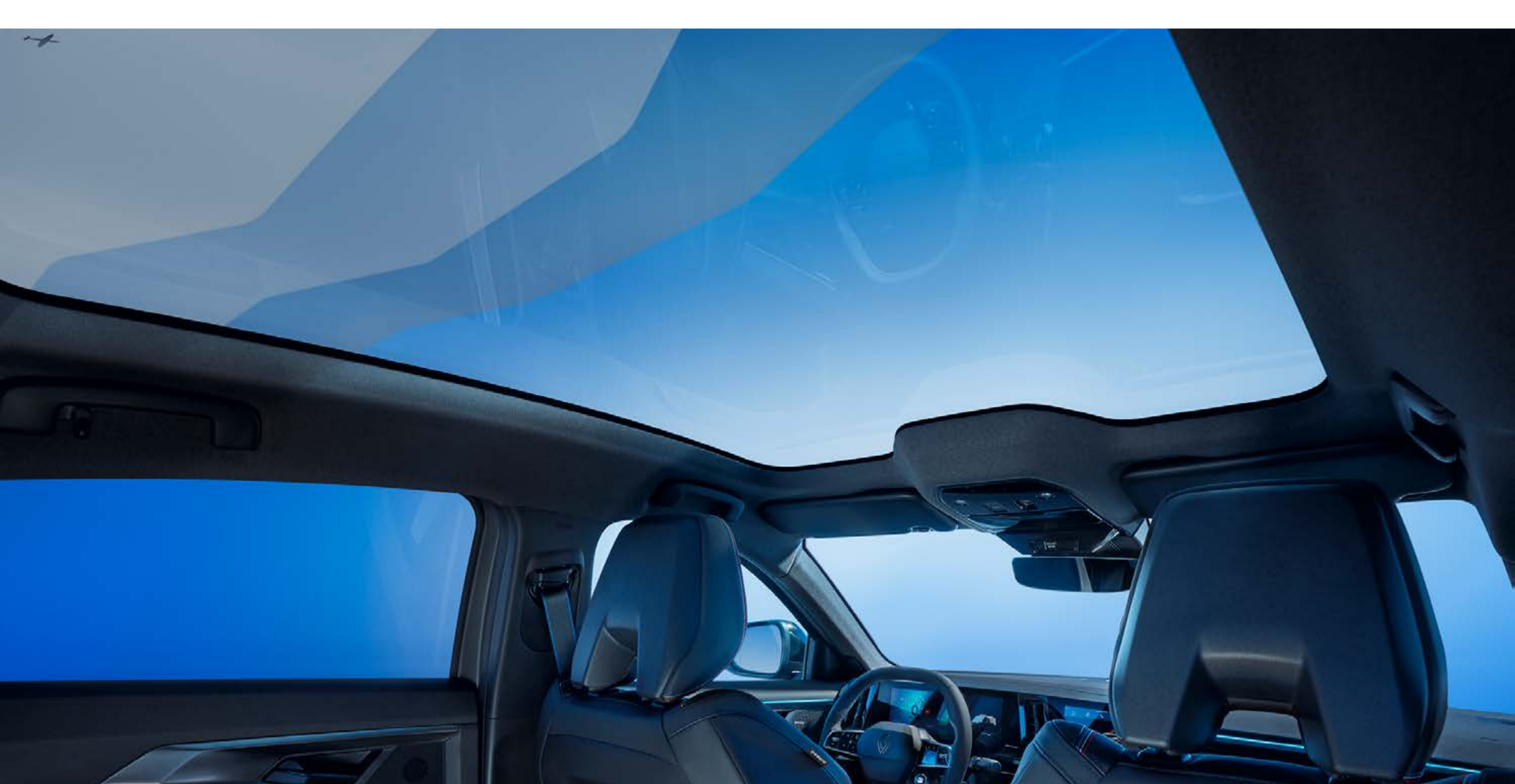
adjustable opacification with 4 modes (open/closed) and 2 zones (front/rear)
