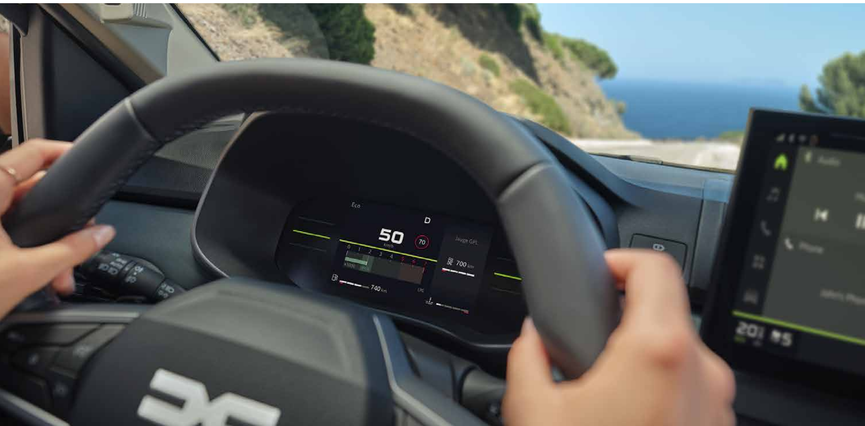
7" digital driver display with driving mode information (3)
