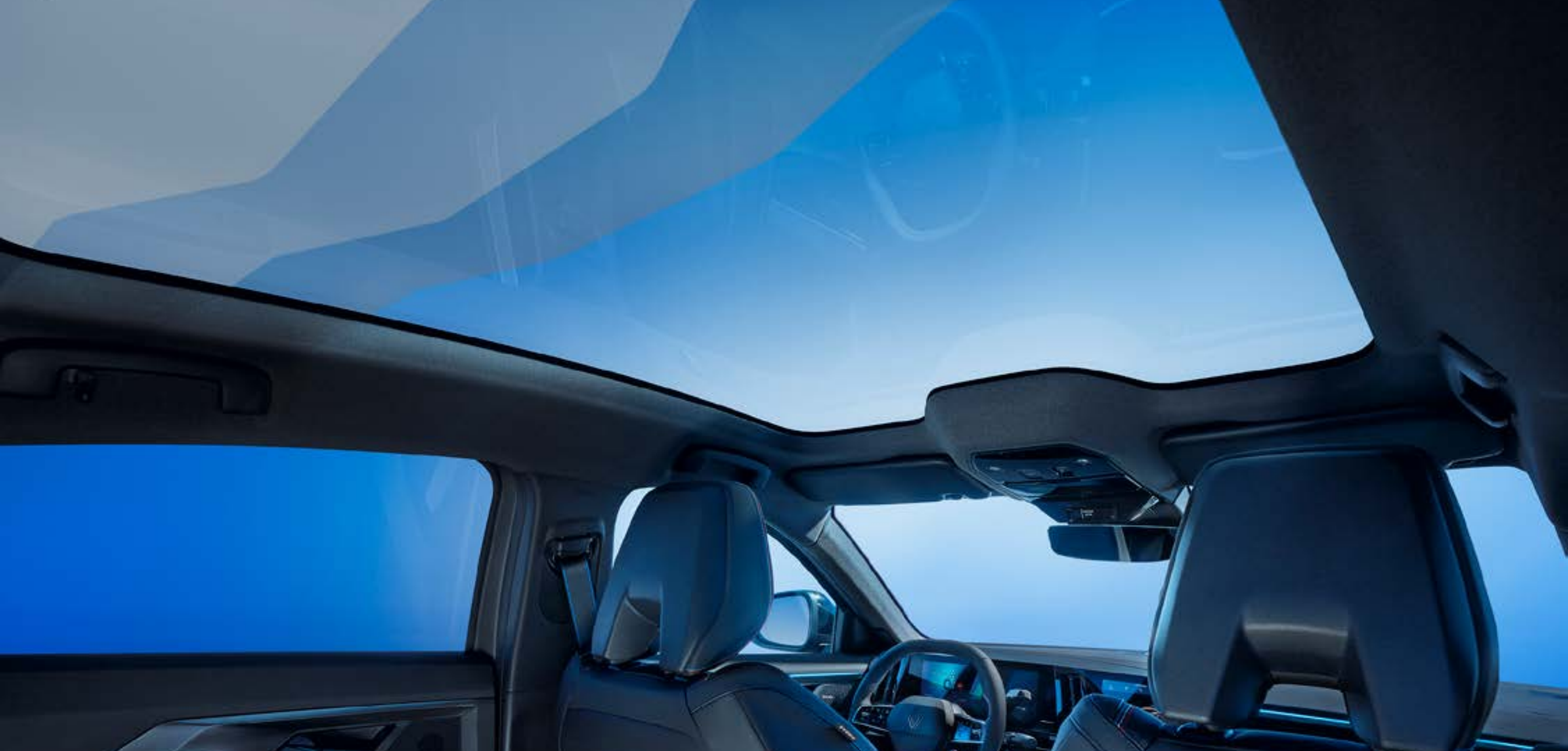
adjustable opacification with 4 modes (open/closed) and 2 zones (front/rear)
