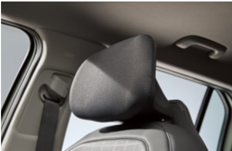
Bio PU foam based on castor oil
