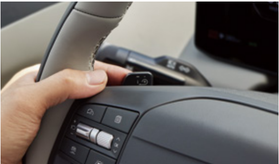
i-PEDAL 3.0 At all stages of regenerative braking, the accelerator pedal can be used to adjust the car's speed or stop it. A memory function is available for reverse parking and restarting. Frosted Blue (EBB) / Specifications above may vary by trim level, engine and options. ※ The reverse parking function can be switched on or off in the system settings menu.
