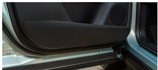
Interior door protection
