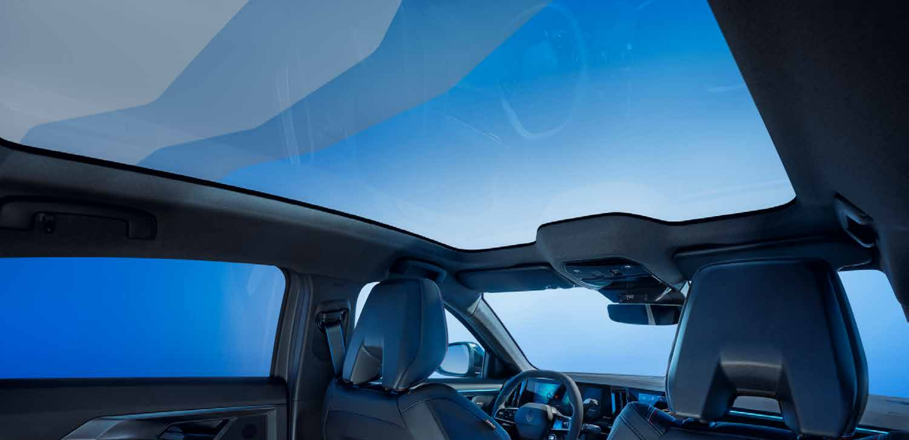
adjustable opacification with 4 modes (open/closed) and 2 zones (front/rear)
