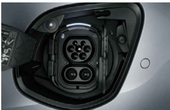
CCS rapid charging port, 80kW max. capacity.
