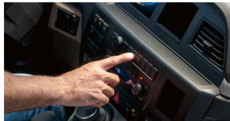
Freely programmable direct access buttons fitted with touch sensors
