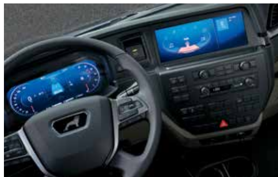
Infotainment system with 12-inch display and control system below the secondary display
