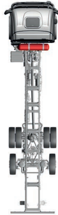
CNG tanks behind the cab, available in combination with: • Left side CNG; right side CNG • Left side CNG; right side free • Left side free; right side CNG
