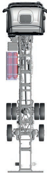
CNG tanks on the left side, available in combination with CNG or LNG tanks on the right side.
