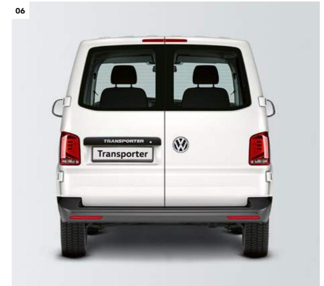
**05 Rear wing doors.** Standard on panel van models and any model ordered with a high roof. | S | H | high roof kombi crew van only. | S | H | panel van.
