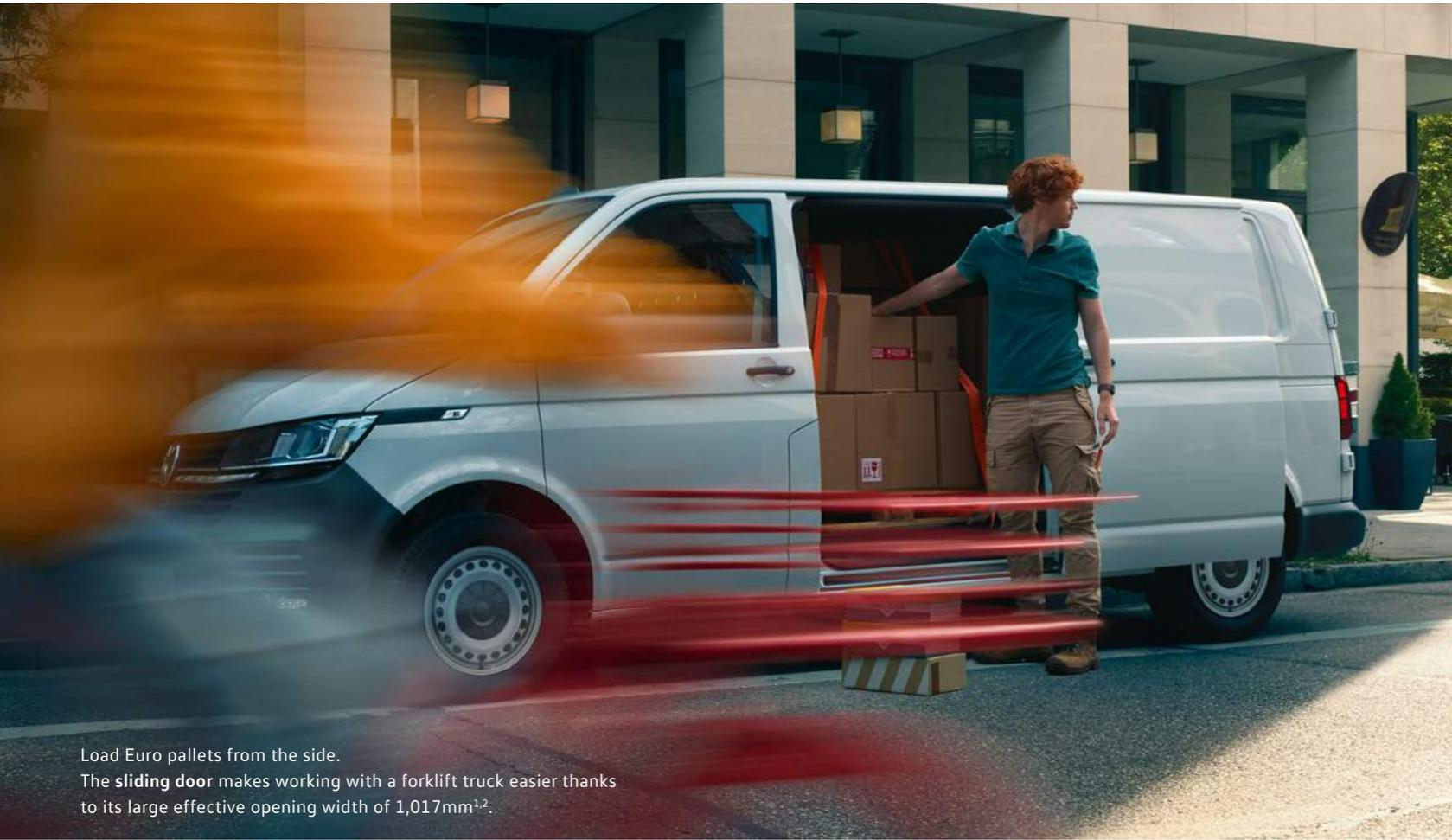
Load Euro pallets from the side. The **sliding door** makes working with a forklift truck easier thanks to its large effective opening width of 1,017mm<sup>1,2</sup>.
