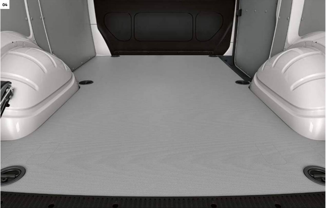
**04 Universal floor (for fittings).** The ideal preparation for subsequent installation of cabinet systems from various manufacturers<sup>3</sup>. Special adapters<sup>4</sup> in the recesses in the floor covering permit flexible installation of cabinet systems at any time without gluing or drilling. Subsequent removal of the floor leaves only minimum traces. Optional on panel van models. |S|H|
