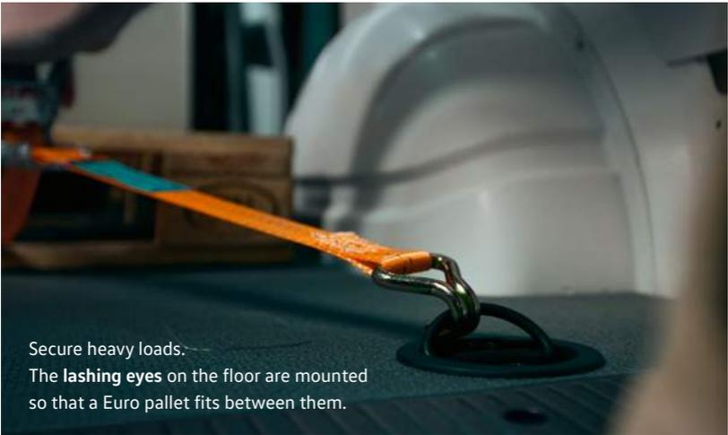
Secure heavy loads. The **lashing eyes** on the floor are mounted so that a Euro pallet fits between them.
