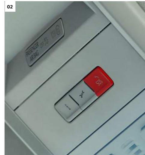
**02 eCall.** Following an accident, automatically sends the time, location and number of vehicle occupants to an emergency call centre and establishes a voice connection. The system is activated by a crash sensor or manually via the emergency call button. If the driver doesn't respond, eCall automatically informs the emergency services. |S|H|
