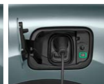
Charging Mode in Progress (Flashing green LED)
