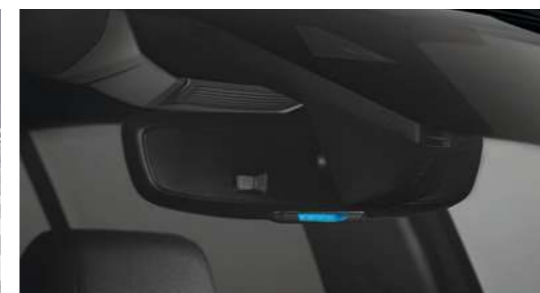
In ZEV mode, a clearly visible blue LED indicator lamp comes on which identifies the vehicle as running in 100% electric mode to other road users.
