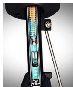
The suspension with Progressive Hydraulic Cushions® succeeds in both filtering and absorbing the unevenness of the road, while ensuring remarkable dynamism.
