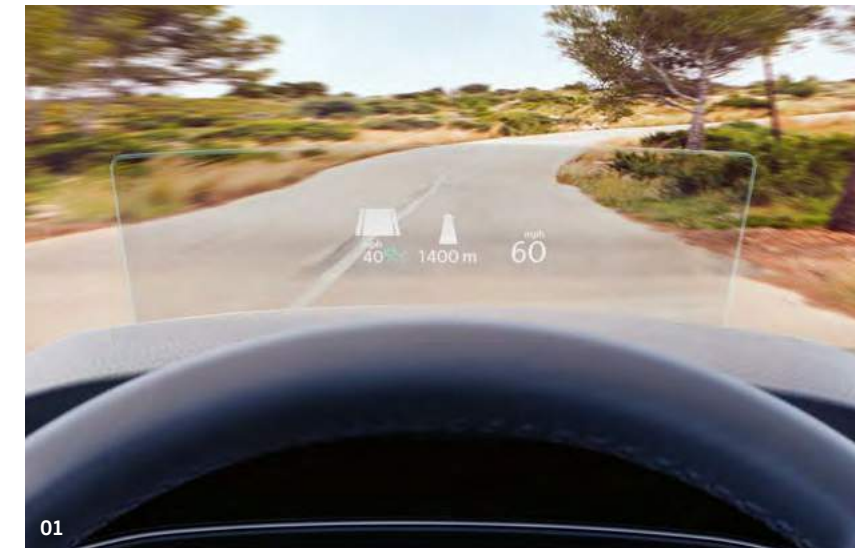
01 The optional Head-up Display 1 presents driving information directly in your field of vision. Speed, traffic signs and information about the assistance systems, as well as warnings and navigation data are projected on to the high-quality retractable screen transparently displayed in front of the windscreen, enabling you to read everything clearly while keeping your focus on the road ahead. Optional on SEL, R-Line, GTE and GTE Advance models.
