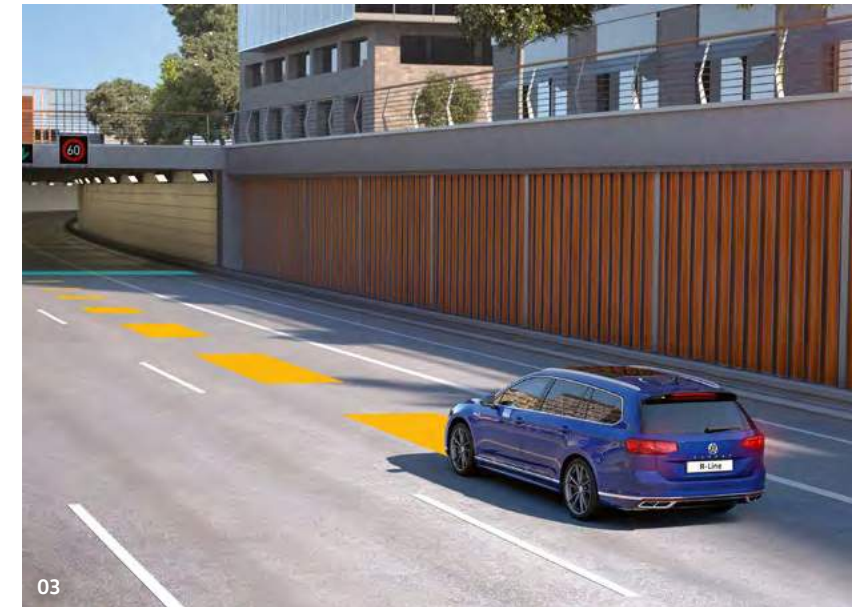
03 Adaptive Cruise Control (ACC) is a radar sensor controlled distance monitoring system that utilises a front mounted camera to set a distance to the vehicle in front and maintain it up to a predetermined set speed by automatically accelerating and braking as necessary. The system adds speed and cornering assistance by using information from the vehicle's navigation system if fitted. Standard on all models.
