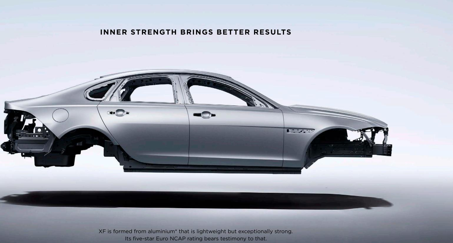
\*Up to 75 percent aluminium content based on volume for body structure excluding doors, bonnet and tailgate.
