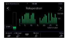
Recuperation is also used to recharge the battery during phases of coasting.
