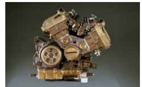
The first Honda V4 engine developed in 1978 for the Road Racing World Championship
