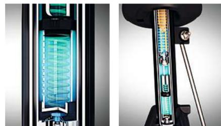
The suspension with Progressive Hydraulic Cushions® succeeds in both filtering and absorbing the unevenness of the road, while ensuring remarkable dynamism.
