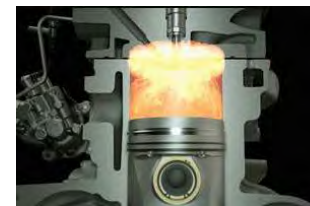
1. 2000 bar High Pressure Fuel System
