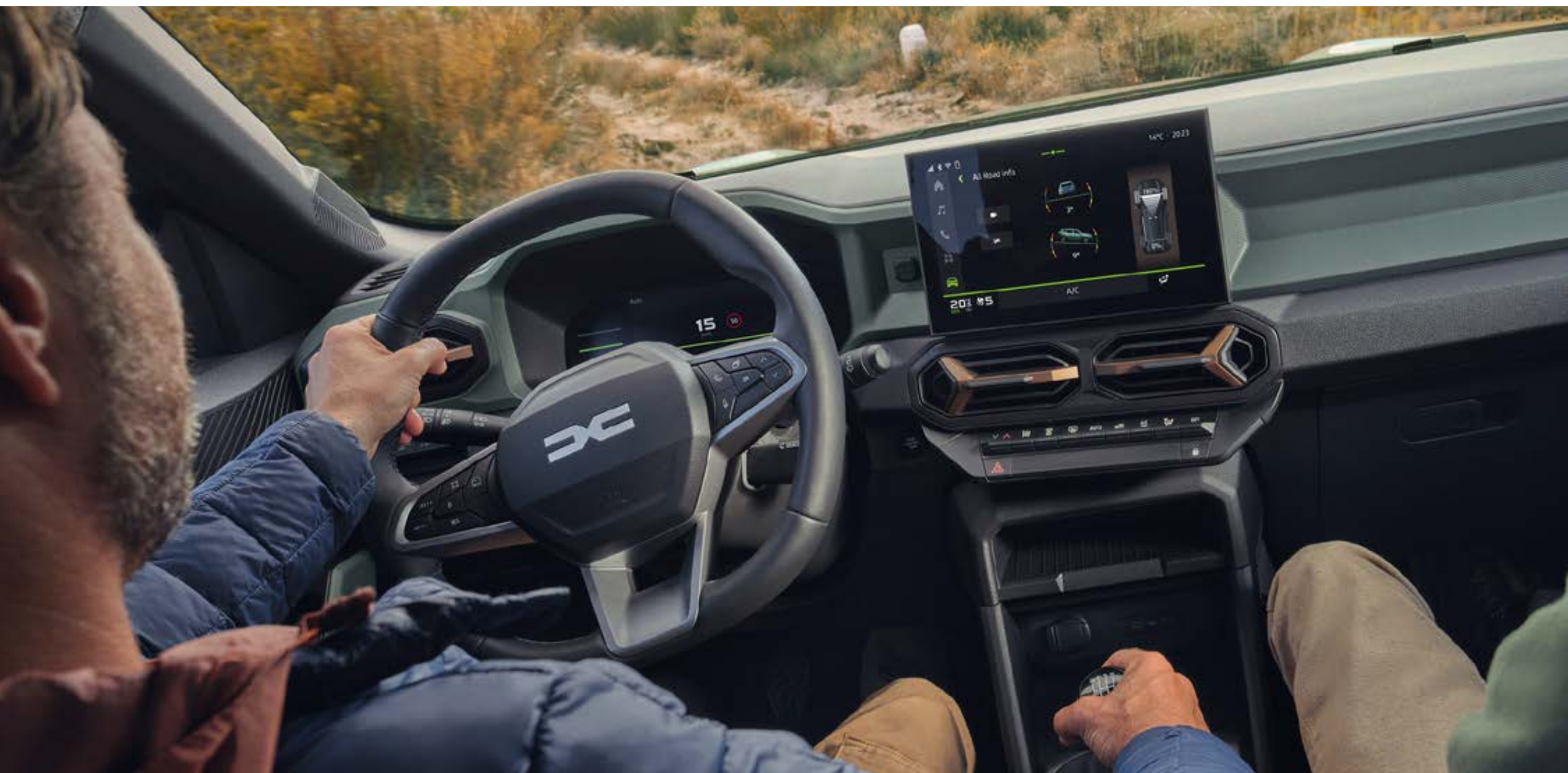
Touchscreen with 4x4 information: slope angles and power per axle
