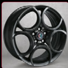
6G6 - 18" 5 hole design alloy wheels with dark finish with 225/40 R18 tyres
