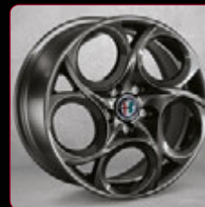
6Y8 - 17" 5 hole design alloy wheels with dark finish with 225/45 R17 tyres
