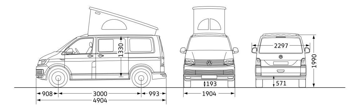
Please note: Vehicle drawings are not to scale. All dimensions in millimetres (mm), unless otherwise stated. The height measurements listed may vary by  $\pm$  50mm depending on model and equipment fitted.
