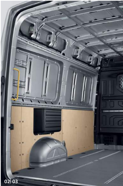
02 Half-height plywood side lining. 1 The load compartment cladding made of 5mm thick rigid plywood panels is especially robust. It is fitted from the floor up to the load-lashing rails and is also highly durable.
