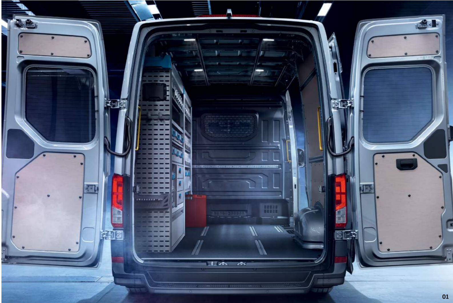
01 Rear wing doors. The two roof-height doors provide an opening angle of 180°. On Trendline models the standard rear wing doors are extended to an increased opening of 270°. The 270° rear wing doors are available as an option on Startline models.
