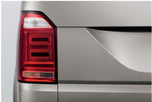
Standard low energy LED tail lights.
