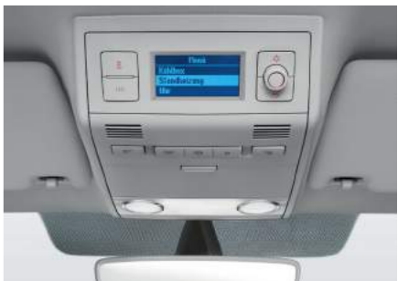
Control unit for the Caravelle's optional auxiliary heater with programmable parking function, remote control and second battery.
