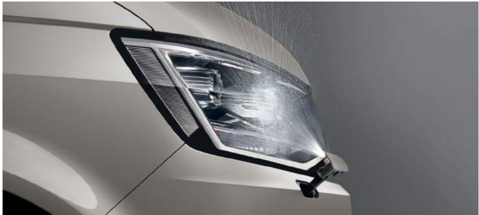
Optional heated headlight washer system.
