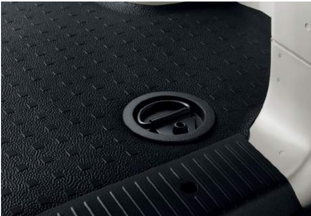
Rubber floor covering with securing points throughout rear passenger area and load compartment.
