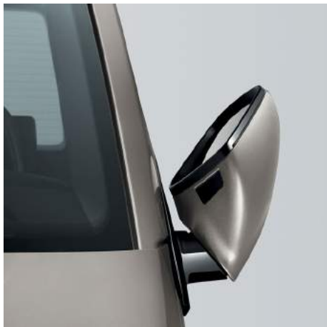
Optional body-coloured electrically adjustable and power folding wing mirrors.
