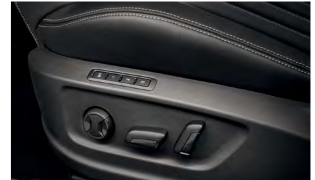
ELECTRICALLY ADJUSTABLE FRONT SEATS WITH MEMORY FUNCTION
