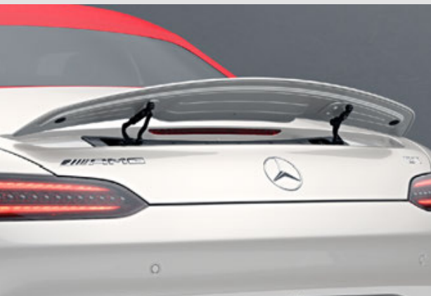
Rear aerofoil – electrically extending
