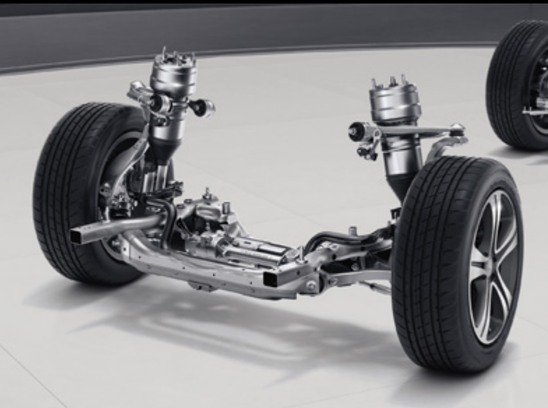
AIR BODY CONTROL – multi-chamber air suspension with continuously-adjustable damping to improve ride comfort and driving dynamics
