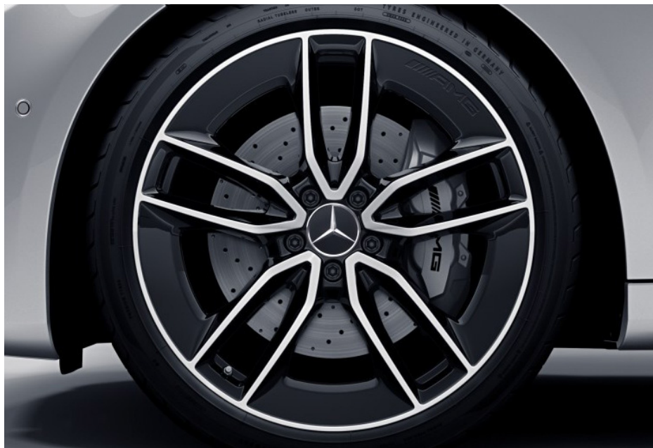
RTZ 20" AMG alloy wheels (4) – 5-twin-spoke design, painted black with high-shine finish front: 245/35 tyres; rear: 275/30 tyres
