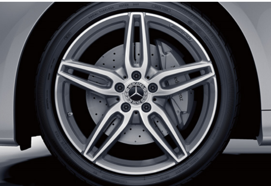
RTD 19" alloy wheels (4) – 5-twin-spoke design, painted titanium grey with high-shine finish front: 245/40 tyres; rear: 275/35 tyres
