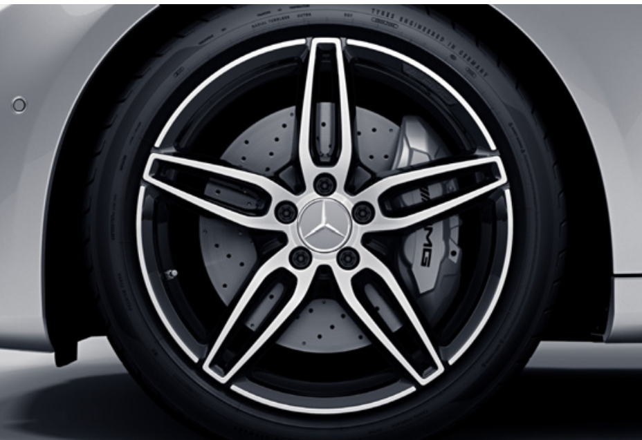
RTE 19" AMG alloy wheels (4) – 5-twin-spoke design, painted high-gloss black with high-shine finish front: 245/40 tyres; rear: 275/35 tyres
