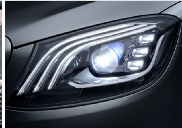
MULTIBEAM LED with ULTRA RANGE Highbeam
