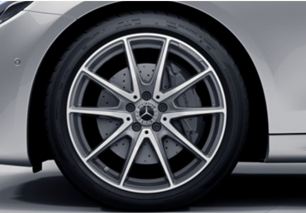
RRD 19" AMG alloy wheels (4) – 10-spoke light-alloy wheels front: 245/40 tyres; rear: 275/35 tyres
