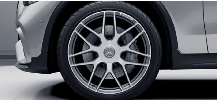
RWD 21" AMG alloy wheels (4) – cross-spoke design, painted titanium grey with a high-shine finish front: 265/40 tyres; rear: 295/35 tyres
