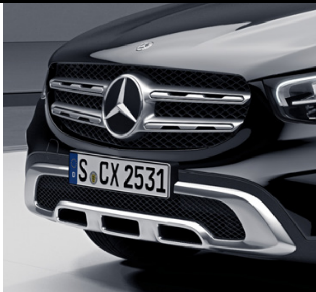
Radiator grille with integral Mercedes star and two louvres in matt iridium silver with chrome inserts
