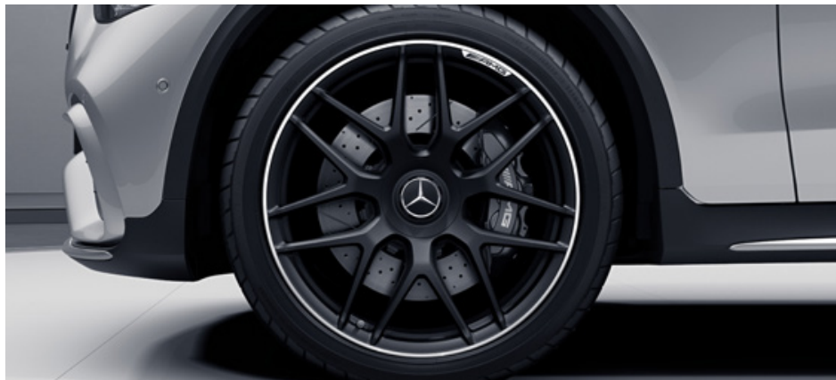
RWE 21" AMG alloy wheels (4) – cross-spoke design, painted black with a high-shine rim flange front: 265/40 tyres; rear: 295/35 tyres
