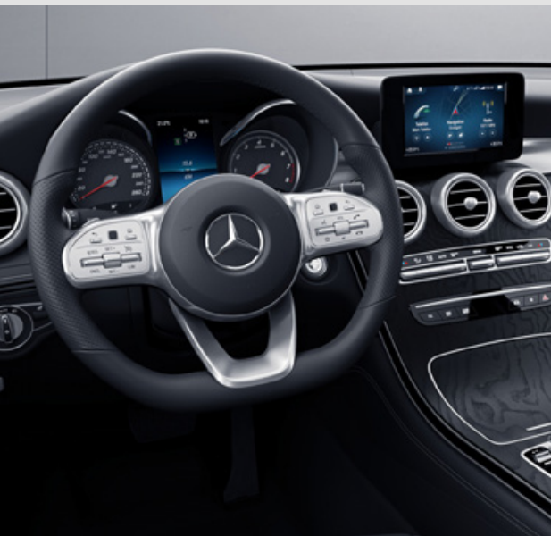
Flat-bottomed steering wheel with touch control buttons
