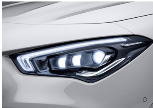
MULTIBEAM LED headlamps with Adaptive Highbeam Assist Plus
