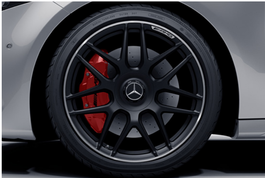
RSZ 19" AMG forged alloy wheels (4) – cross-spoke design, painted matt black with a high-sheen rim flange 255/35 tyres
