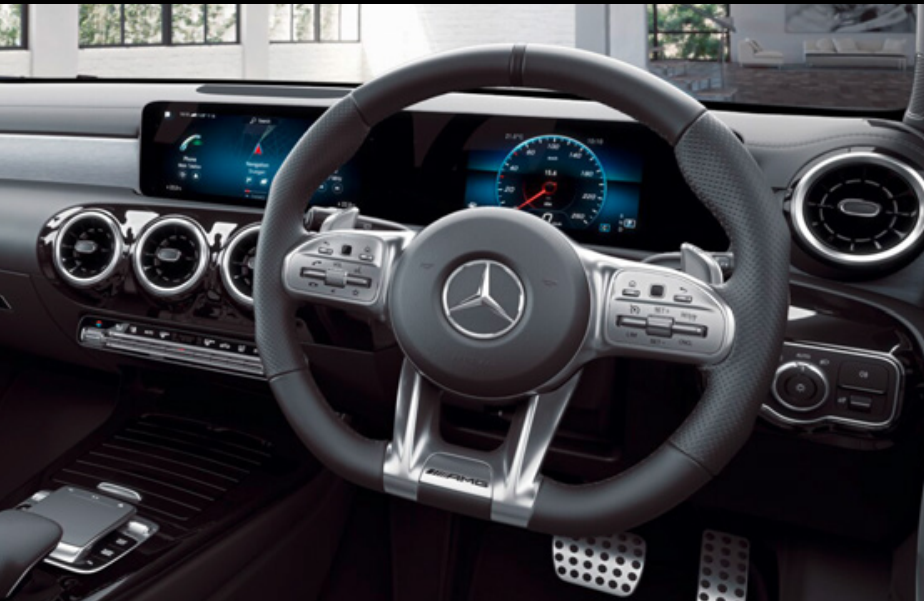
7-inch digital instrument display and a 10.25-inch touchscreen media display
