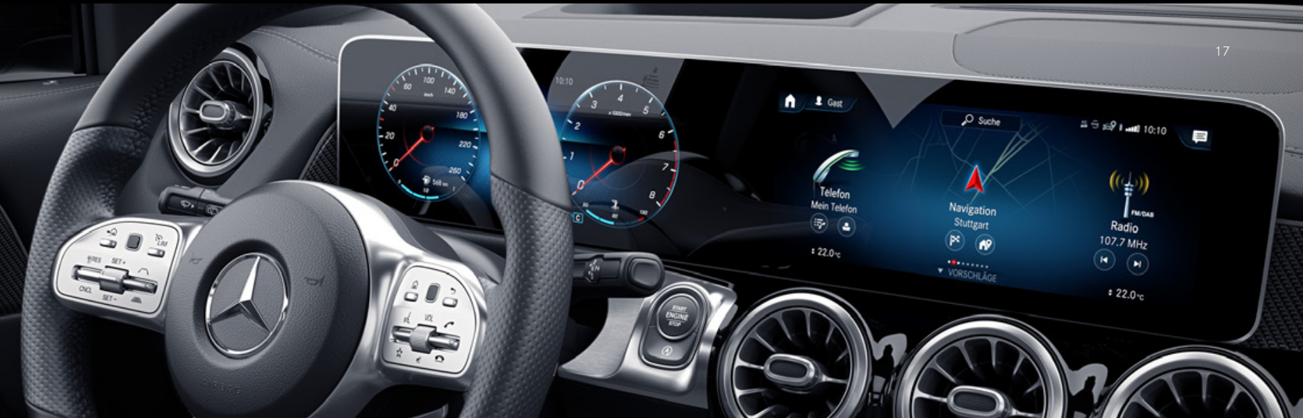
10.25-inch digital instrument display and touchscreen media display
