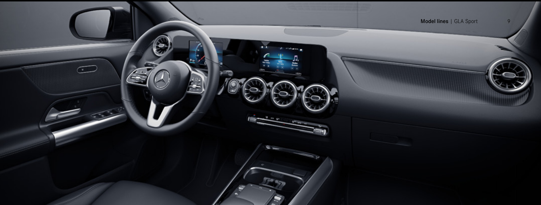
7-inch digital instrument display and 7-inch touchscreen media display
