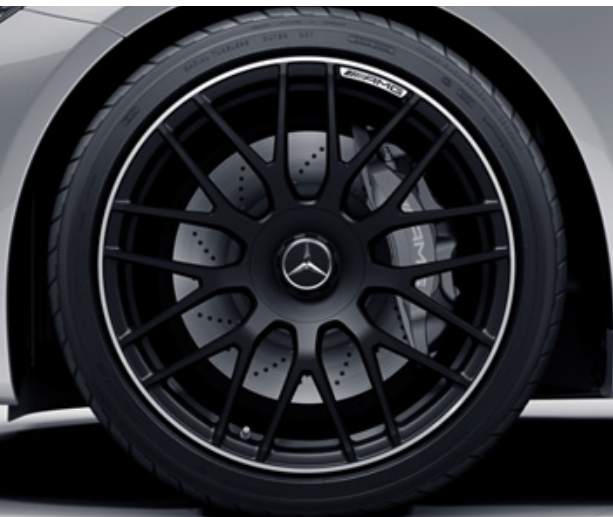
767 19"/20" AMG alloy wheels (4) – forged cross-spoke design, painted matt black front: 255/35 tyres; rear: 285/30 tyres
