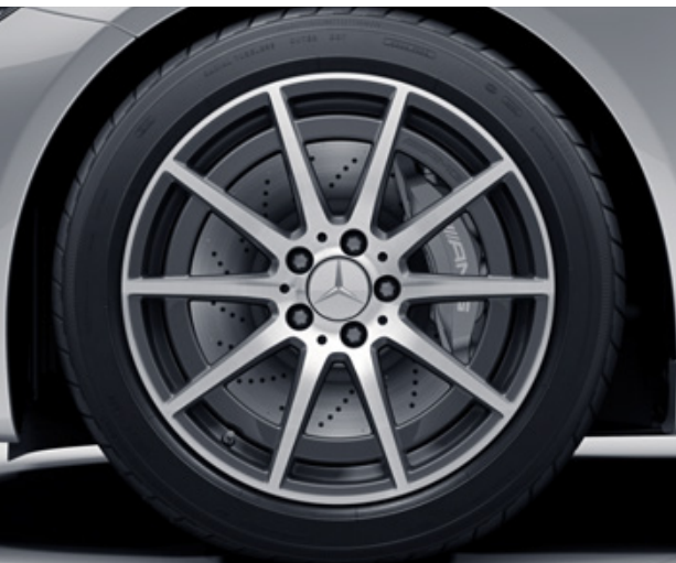
RUP 18" AMG 10-spoke alloy wheels (4) – aerodynamically optimised, painted tantalite grey with a high-sheen finish front: 245/40; rear: 265/40
