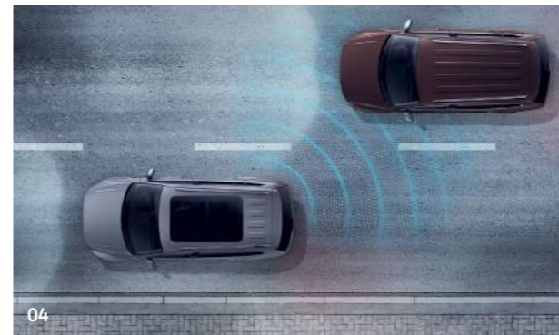
04 Side Scan provides assistance if you want to change lanes from speeds of 37mph upwards. Sensors in the rear of the vehicle monitor the traffic and should they detect any road users in your blind spot or vehicles approaching quickly from behind, the system will alert you via a warning light within the door mirror housing and an audible warning within the vehicle. The parking assistant monitors the area behind and next to your vehicle, alerting you if it detects a vehicle or object, and automatically instigating an emergency stop if a collision is imminent. Optional on all models.
