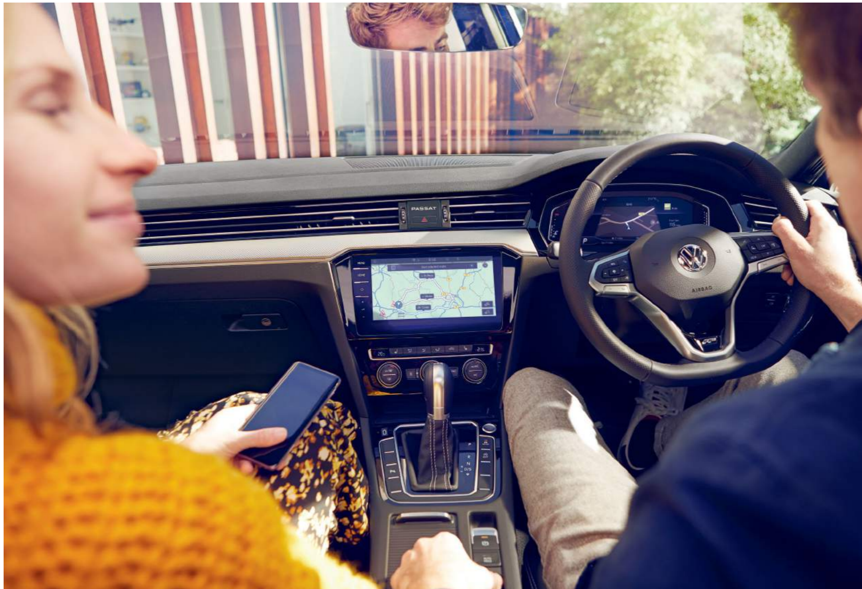
01 The optional Head-up Display 1 presents driving information directly in your field of vision. Speed, traffic signs and information about the assistance systems, as well as warnings and navigation data are projected on to the high-quality retractable screen transparently displayed in front of the windscreen, enabling you to read everything clearly while keeping your focus on the road ahead. Optional on SEL, R-Line, GTE, GTE Advance and Alltrack models.
