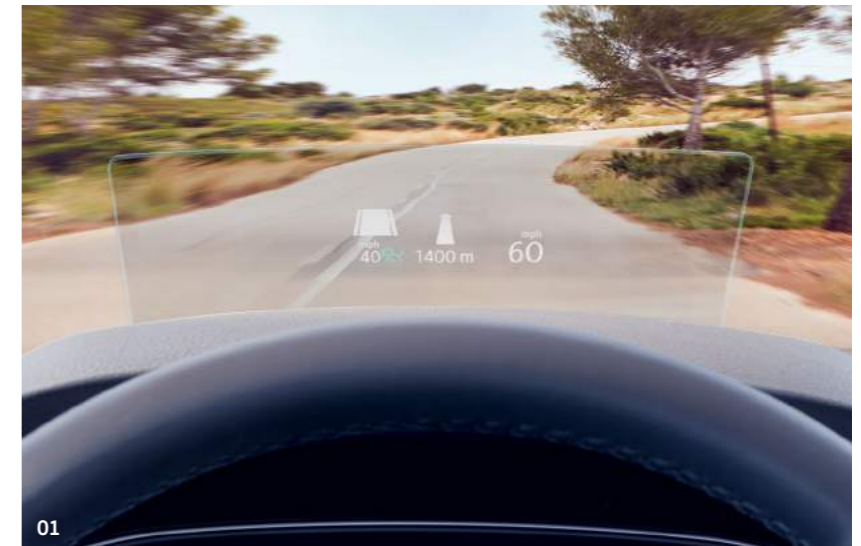
01 The optional Head-up Display 1 presents driving information directly in your field of vision. Speed, traffic signs and information about the assistance systems, as well as warnings and navigation data are projected on to the high-quality retractable screen transparently displayed in front of the windscreen, enabling you to read everything clearly while keeping your focus on the road ahead. Optional on SEL, R-Line, GTE, GTE Advance and Alltrack models.
