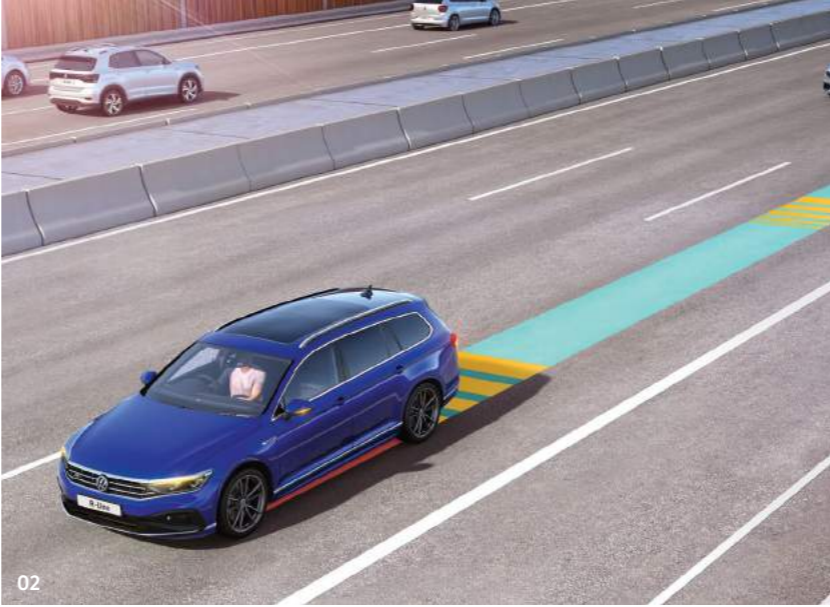
02 Emergency Assist can help even further should a driver medical emergency situation arise. In conjunction with the DSG gearbox, the system recognises an incapacity of the driver and slows the car down in its lane to a standstill if necessary. As soon as the system cannot detect any steering, braking or acceleration activity, it alerts the driver. If the driver remains inactive, it automatically activates the hazard warning lights to alert other road users. Standard on all models in conjunction with the DSG gearbox.
