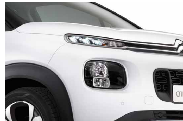
Halogen headlights with LED Daytime Running Lights
