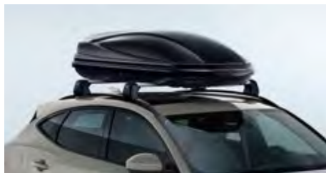
Roof Luggage Box Spacious 410 litre capacity lockable roof luggage box, measuring 175 x 82 x 45cm.
