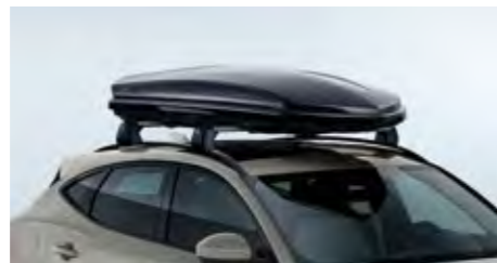
Roof Sport Box Spacious 320 litre capacity lockable roof box designed for sports equipment, measuring 206 x 84 x 34cm.
