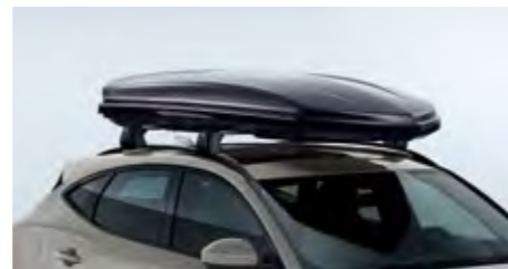
Roof Sport Box - Large Power-click quick mounting system with integrated torque indicator for easy and secure fixing with a single-handed grip.
