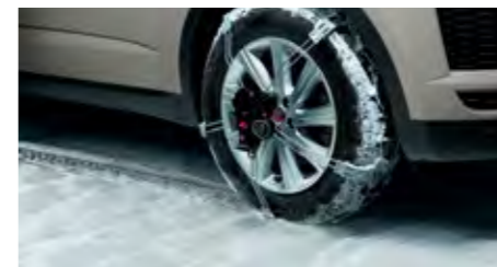
Snow Traction System Improved mobility in snow, mud and icy driving conditions with this high-grip snow chain traction system.
