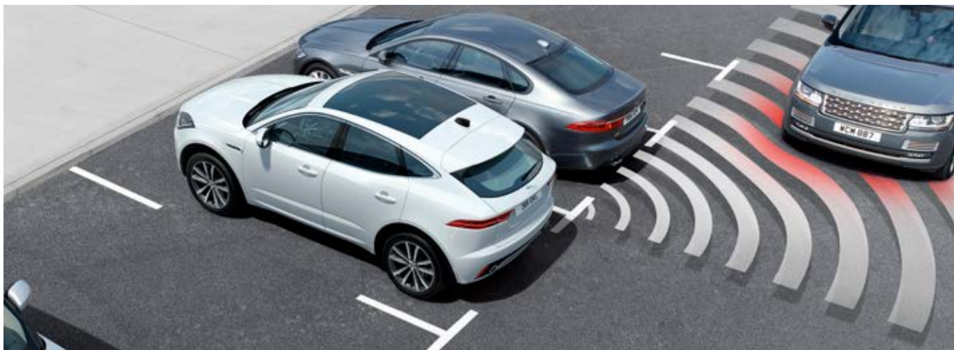
Rear Traffic Monitor
