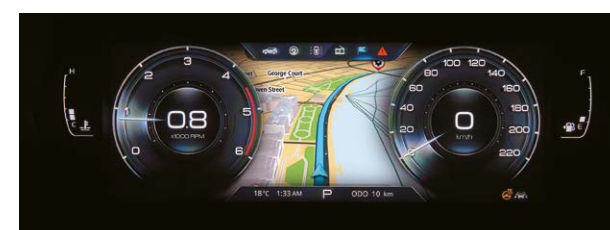
Analogue style instruments with in-cluster navigation
