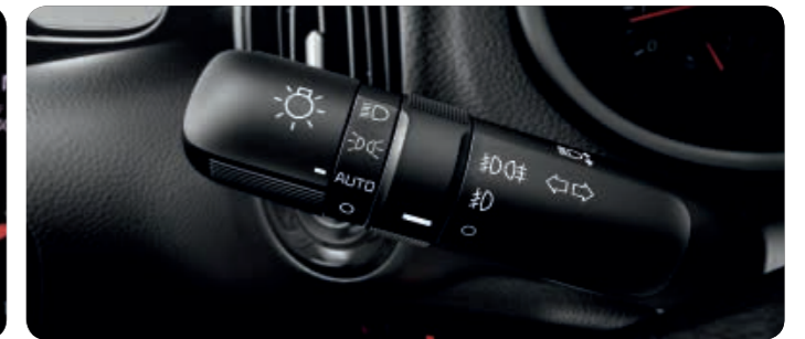
Auto light control Set the stalk ring to Auto and the front and rear lights will turn on or off depending on lighting conditions.
