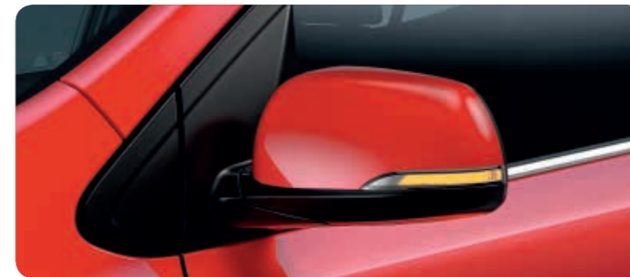
Body coloured exterior mirrors Get a more luxurious look with body-coloured exterior mirrors. They are also heated and have a folding functionality with stylish integrated LED indicators.
