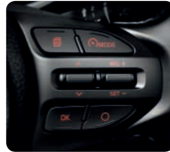
Auto cruise control and speed limiter Set, adjust or cancel the automatic system, with buttons right at your fingertips.
