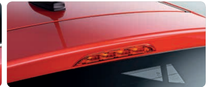
High-mounted stop light From the subtle spoiler above the rear window, the high-mounted stop light helps drivers behind you see when you're braking.
