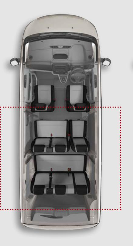
Second-row, two-seat bench with a folding seat and a third-row, three-seat fixed bench with up to c1.2cu.m of usable loadspace.
